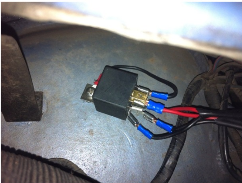
The left hand relay on the inner guard, just near the DB10 Flasher relay.
