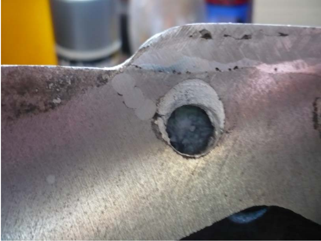
First crack repaired 1999
