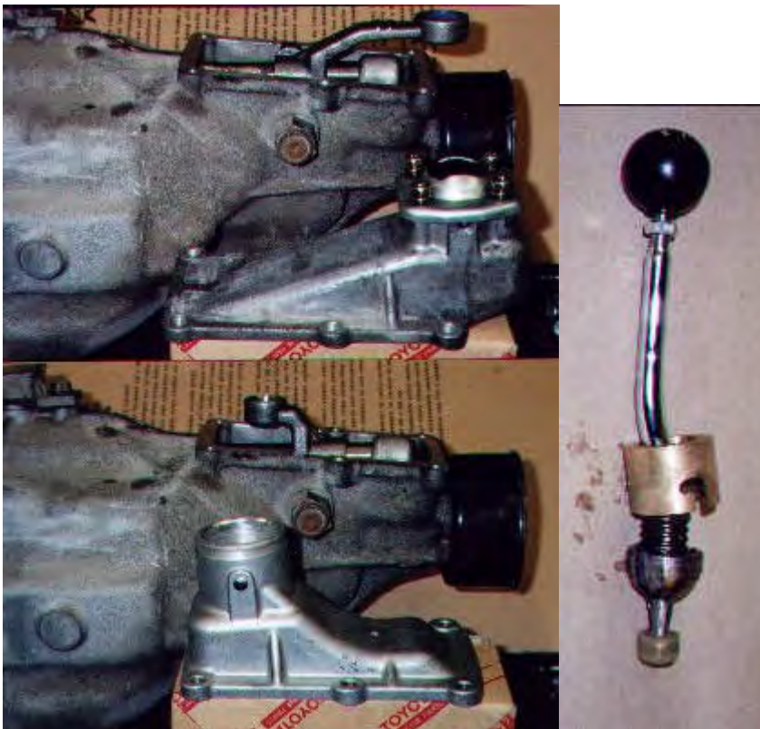
Illustration of the two lever positions, standard Supra, top, and as Healey centre change bottom. Also lever with new brass retaining bush.
