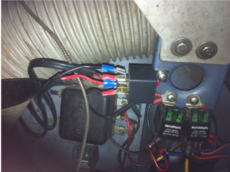
The right hand relay on the shroud support together with the Fog & Driving, Headlight & Horn relays.
