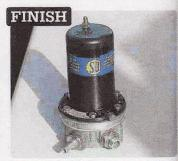
It's alive! One reconditioned fuel pump. If the points fail prematurely I'll consider upgrading to the electronic kit available, or replacing the pump altogether with a new no-maintenance electronic version. But for now the engine starts first time. Job done.
