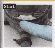
Check the pump you have fitted to your classic is the correct type before you order the rebuild kit. Check the ID tag screwed to the main body. It's not unheard of for the wrong pump to be fitted.
