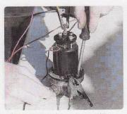
Energise the coil This ensures the diaphragm's in its forward position. Insert an old fibre washer between the lower lug and coil housing.
